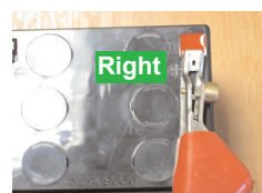
Grip clips tightly around tab terminals
