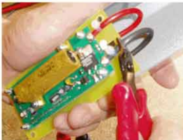
Step 3 Cut and remove old leads.
