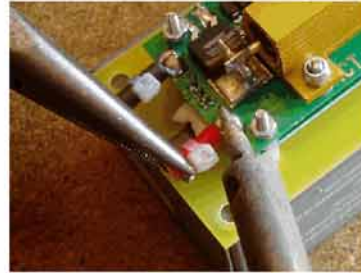
Step 4 Remove lead ends.
