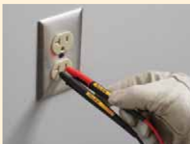
Increase tip exposure for CAT II probing
