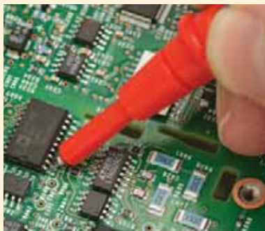
Reduce tip exposure for accurate placement
